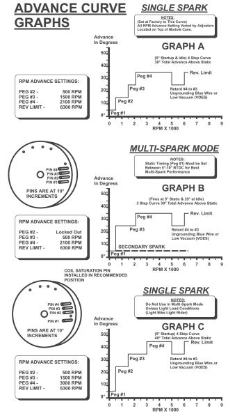
**GRAPH A:** This setting will work with most engines, giving a 30° overall advance above the static timing or an overall timing of 35° at 2100 Rpm's, if static timing is set at 5°. If more advance is needed for top end performance the trigger plate may be rotated clockwise. If pinging is noticed at take off (to much static timing) or static timing exceeds 15° you should use GRAPH C.
