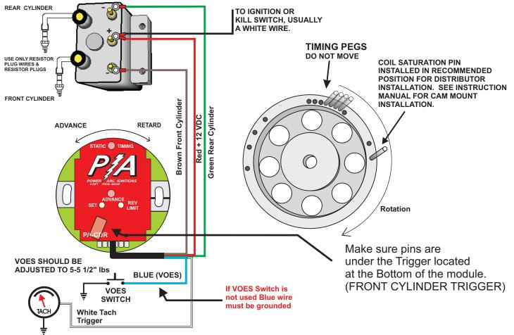
Note: Stock distributor will not work, a distributor that will accept cone mount ignition systems is required.
