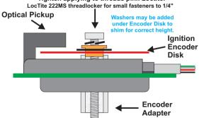
Extra washers may be included for shimming the Encoder Disk outward. Place on encoder standoff if Encoder Disk is to close to Optical Pickup.
