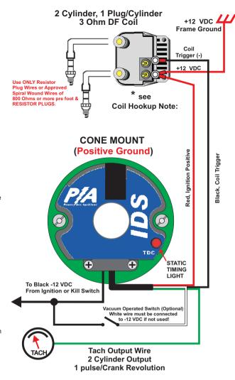
Use of NGK 5K Ohm resistor spark plug boots are recommended when plug wires have less than 2,000 ohms of resistance, resistor spark plugs are still required.
